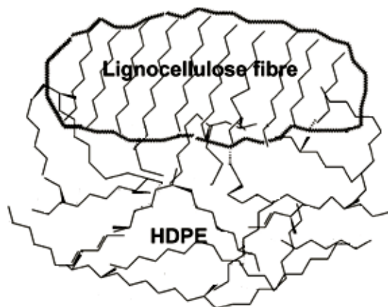
Fig. 3. Adhesion mechanism for lignocellulosic material and HDPE (modified from Colom et al. , 2013).
