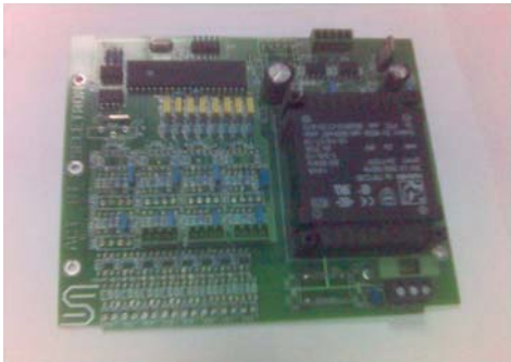
Fig. 8 The digital recording module using the microcontroller with integrated Port-A analog-digital converter
